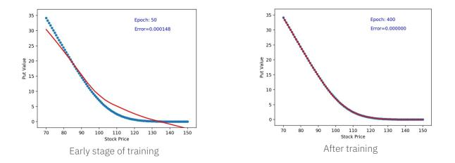
A simple example of DNN training on a put option value function. The blue dots represent training data generated by traditional models. The red line in a DNN approximation. After training, DNNs become smooth, very accurate and very fast approximators.
